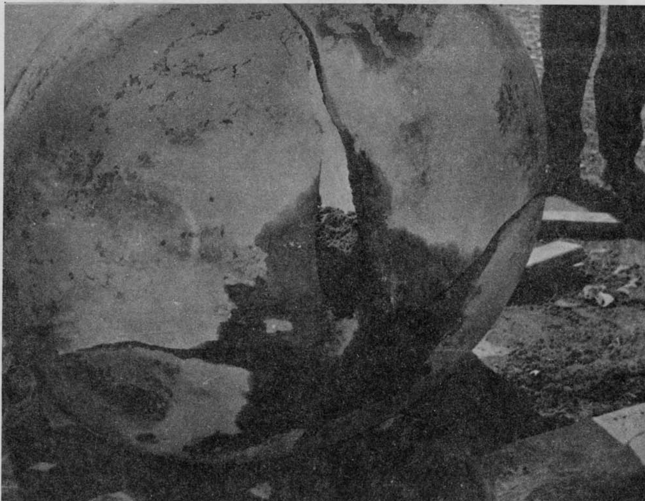
Figure 12. Cracks in Bottom of Liner After Test Using 6 Pounds of TNT Explosive
