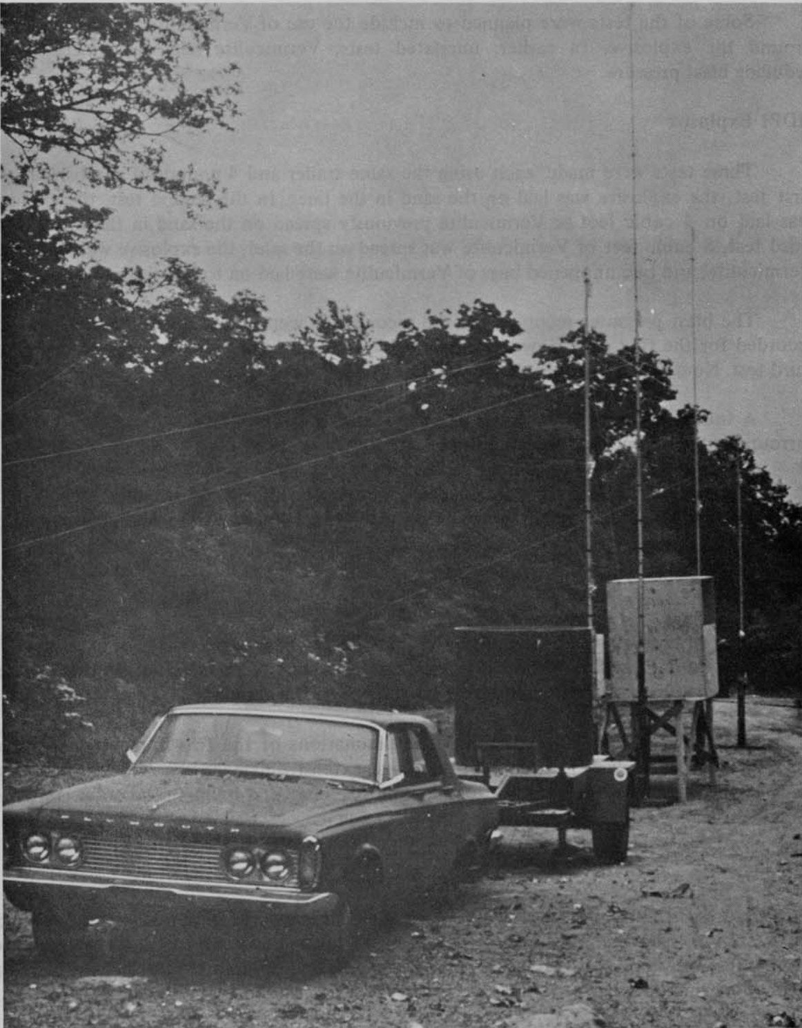
Figure 13. General View for Trailer Tests Showing 4 Door Sedan, Trailer, Simulated Truck Cab and Blast Gage Instrumentation
