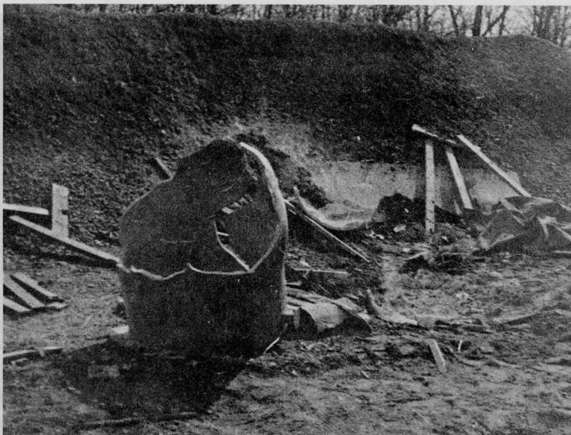
Figure 11. Fracture of Inner Liner After Third Test Using 20 Pounds of HDP1 Explosive
